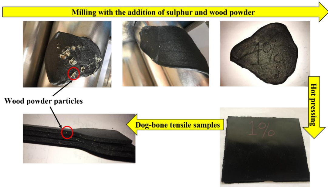
Figure 15 Tensile sample preparation process (1% wood content example)
