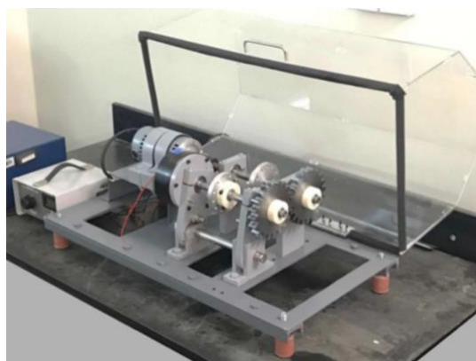
Figure 7. Acquisition test rig system with two gears attached at a QU lab.
