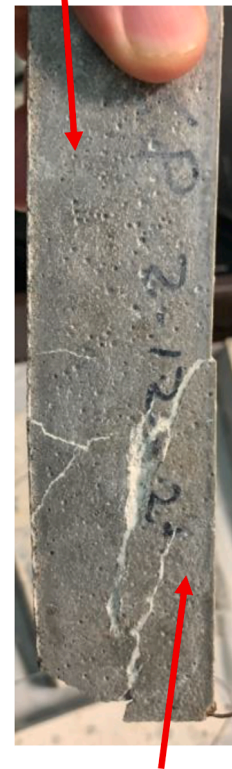
Broken pieces joined together with calcium carbonates
