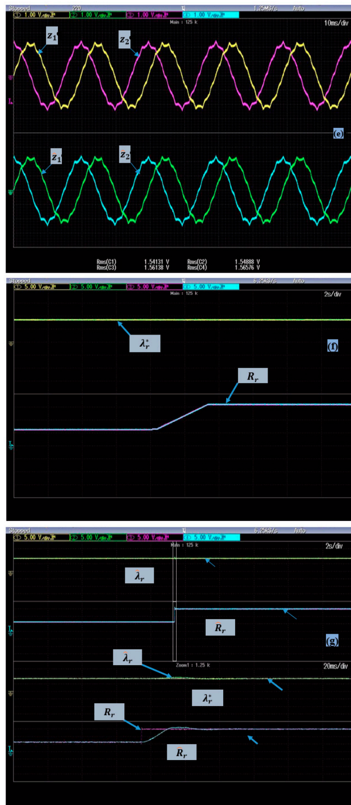
Figure 3. Real time results of sensorless control of five-phase IM drive. (a) Speed, (b) torque, (c) Stator currents (complete view), (d) Rotor flux (Reference and estimated signals), (e) Zoomed view of stator currents (actual and estimated), (f) Rotor flux and rotor resistance variation, (g) Rotor flux dynamics under rotor resistance variation.
