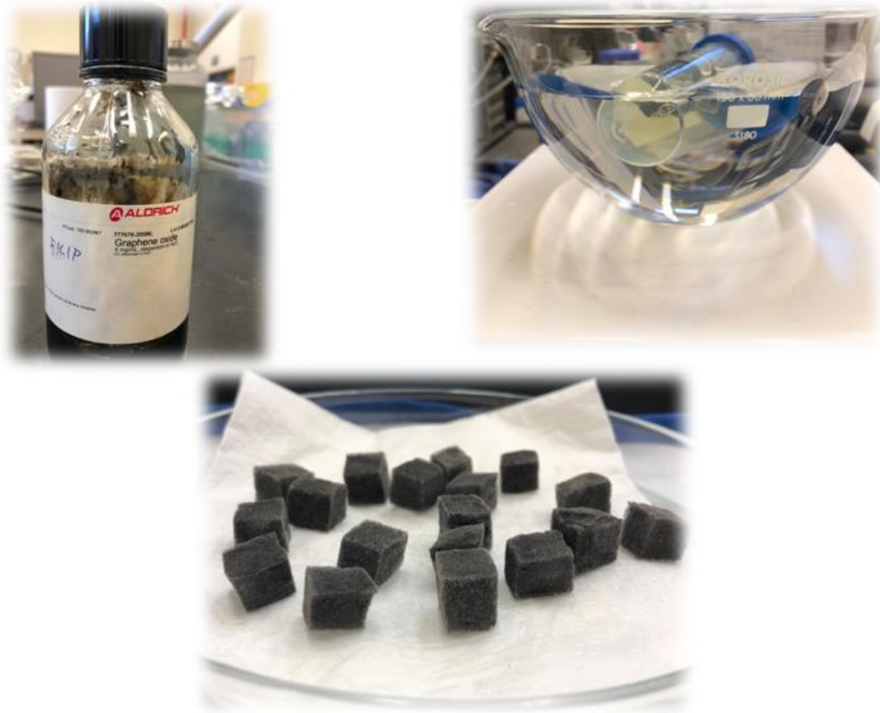
Figure 7: Preparation of melamine foam treated with graphene oxide
