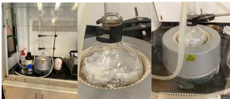
Figure 6: Extraction experiment using xylene
