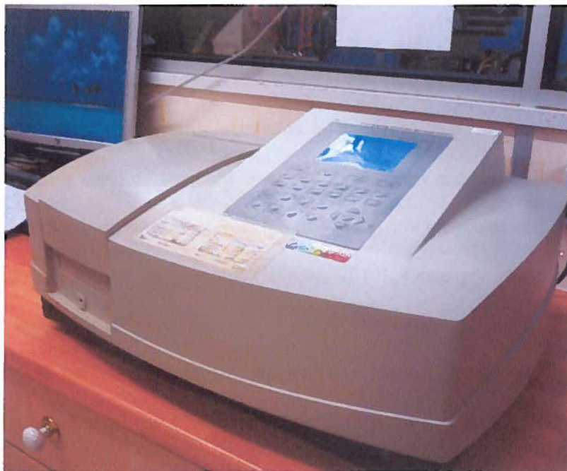
Figure 11 Camspec M550 UV-VIS spectrophotometer which is used in Gradko for the analysis of NO 2
