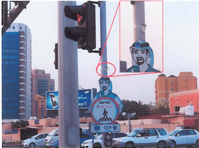
Figure 10 Diffusion tubes mounted on a traffic pole in one of the study area sampling locations
