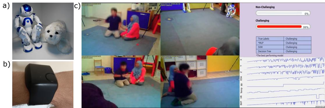
Figure 3.2: An overview of the adopted methodology in this study. a) The two social robots (i.e., Nao and Paro) that were used in this study as part of the stimuli group [65]. b) The wrist wearable device Empatica E4. c) A snapshot of the developed observation and annotation assistive tool during the session with the child when he was exhibiting challenging behaviours during the session with social robots. The tool displays the recorded video, wearable signals acquired from the child, and a summary of the machine learning predictions in real time (See supplementary material).
