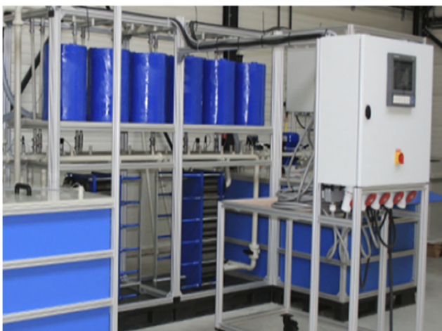
Fig. 9 Aquastill pilot unit [41]
