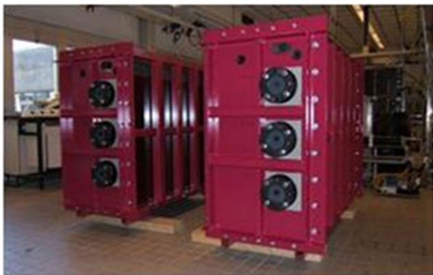
Fig 2 Memstil pilot unit in Singapore [21]
