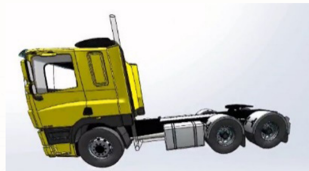
Figure 3. Installation of the smokeless exhaust tube onboard a truck.
