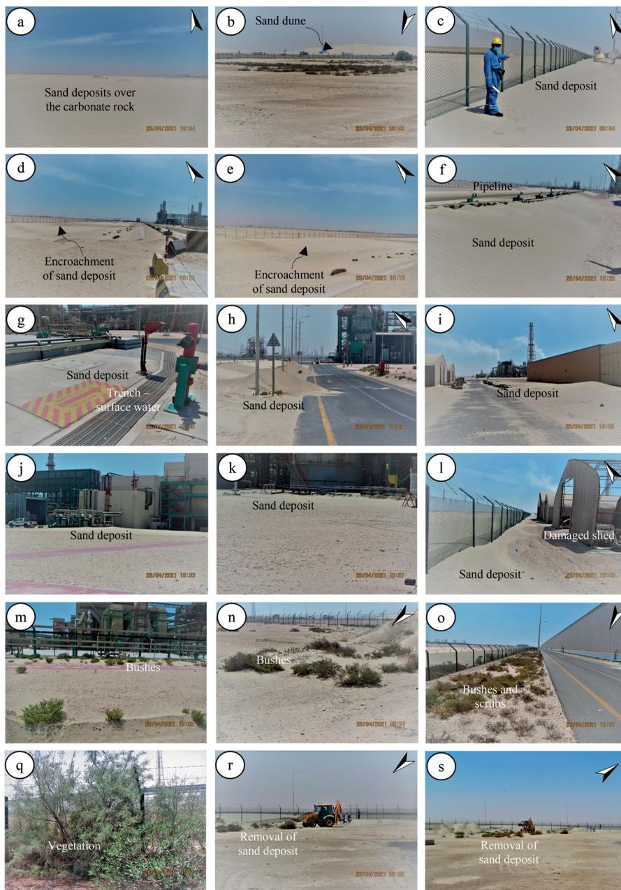
**Figure 7.** Field photographs show (a) the occurrence of sand deposits (b) the sand dune (c) the fences (d) and (e) the encroachment of sand (f) to (i) the sand deposits over the pipeline, water trenches, metal roads (j) and (k) the sand deposit in the industry site (l) the damage of industry shed (m) to (q) the presence of vegetation, grasses and bushes and (r) and (s) the removing of sand deposits along the fences in and around the QAFCO site 5/6. Arrow indicates the direction of the north.
