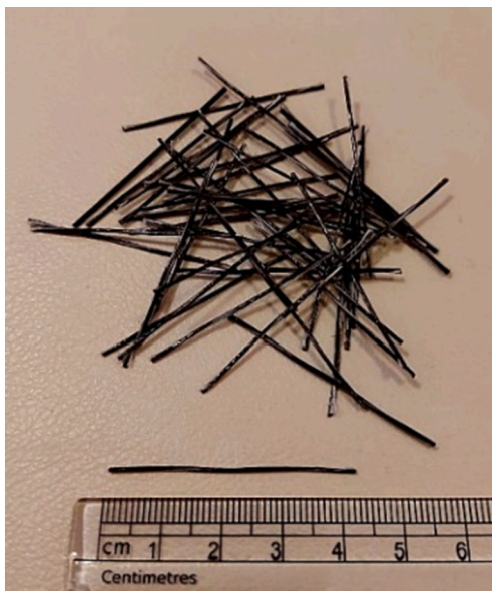
Fig. 4. Basalt macro fibers (BMF).
