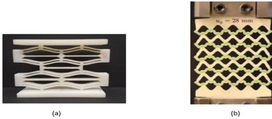
Figure 9. (a) Negative stiffness honeycomb structure [12] and (b) Different metamaterial honeycomb structure under tension [13].
