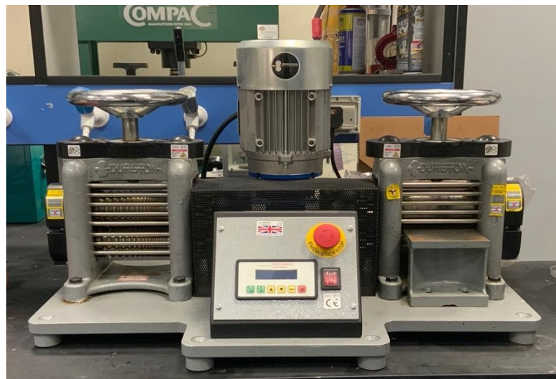
Figure 8: The rolling mill used to roll the samples during thermomechanical treatment.
