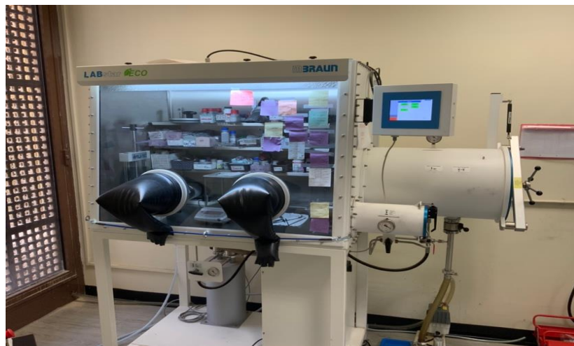
Figure 4: glove box under argon gas
