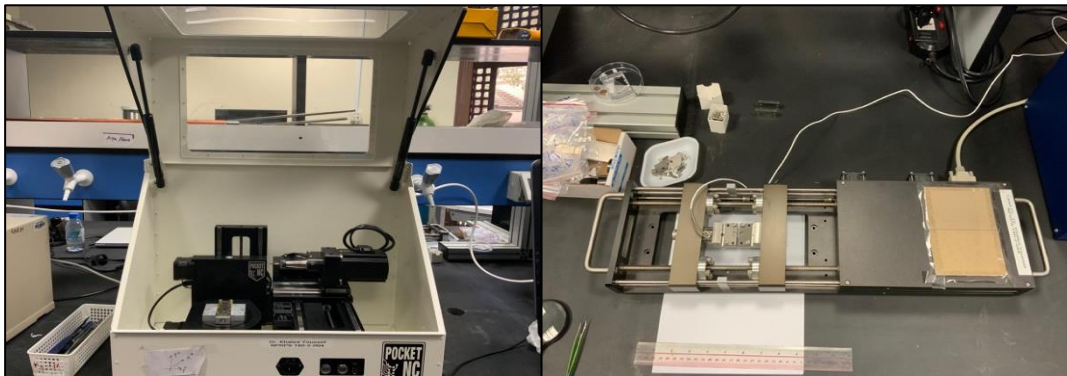
Figure 10: A miniturized tensile machine (MTESTQuattro).
