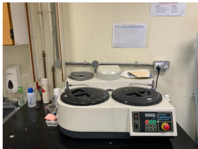
Figure 15: Image of the Polisher (FORCIPOL2V-Metkon)
