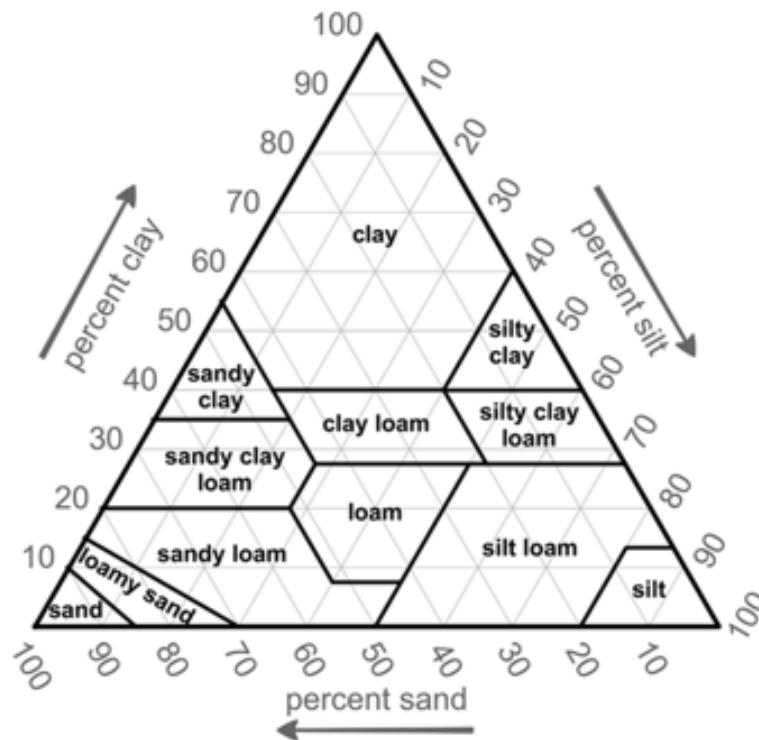
Figure 2. Classes of soil texture according to the particle percentage (Groenendyk et al., 2015)
