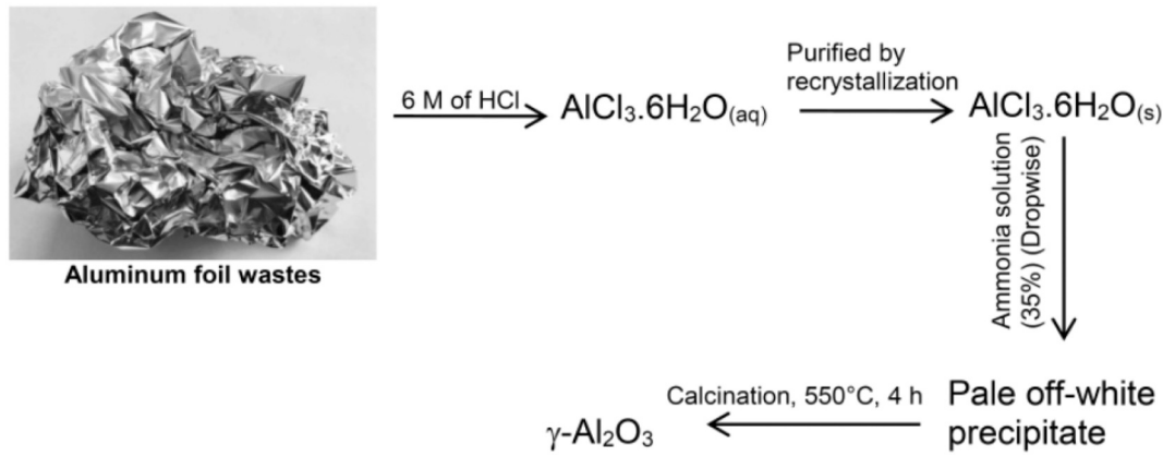
Fig. 1. Proposed schematic illustration of nano- \gamma\text{-Al}_2\text{O}_3 preparation from aluminum foil waste.
