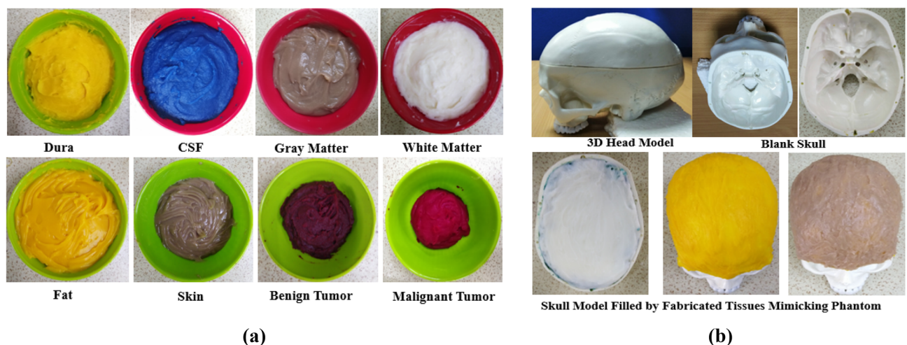
Figure 21. (a) Fabricated six tissue-mimicking phantom layers, including tumors; (b) 3D blank head model and skull model filled by fabricated tissue-mimicking phantom.
