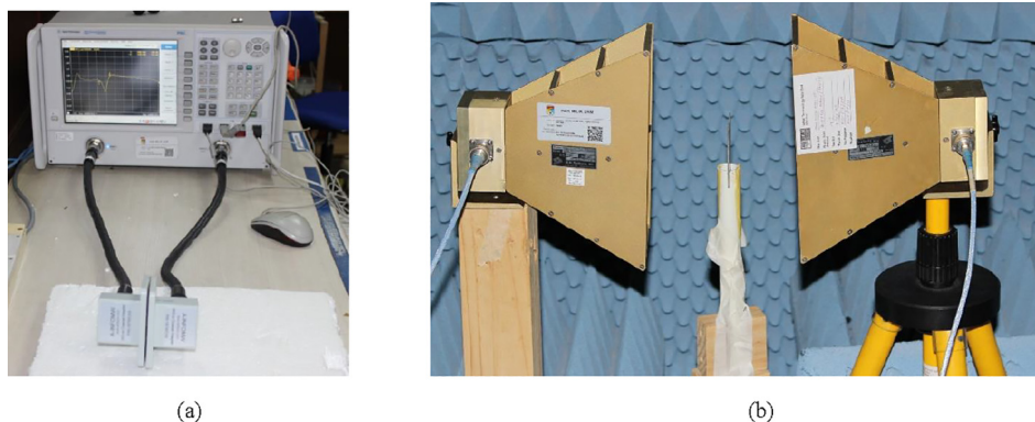
Fig. 27. (a) Measurement set up for evaluating performance of unit cell (b) measurement set up for array.
