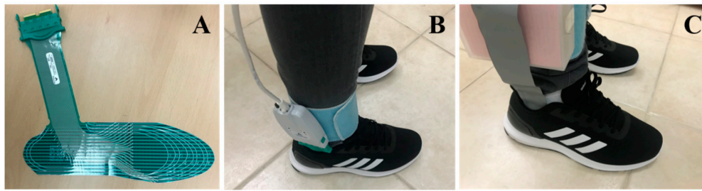
Figure 9. F-scan commercial system (A), F-scan system worn by Subject 01 (B) and FSR-based prototype system worn by Subject 01 (C).
