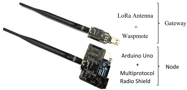
FIGURE 4. LoRa with waspmote and multiprotocol radio shield.
