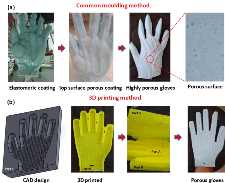
Fig. 3. Fabricating channel embedded elastic gloves and texturing glove surface with porous morphology. (a) Common mold-making method. (b) 3D-printing method.
