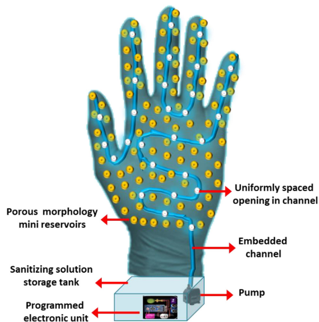
Fig. 1. Schematic representation of reusable self-sanitizing gloves.
