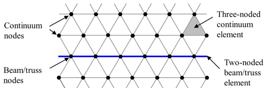
Fig. 2: Concept of the shared or merged nodes
