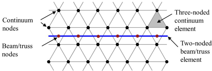
Fig. 3: Concept of the constraint nodes
