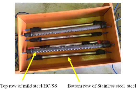
**Fig. 1:** Mold for block samples with a top row with either mild steel/high chromium/stainless steel, and a bottom row with stainless steel only
