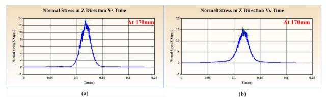
**Fig. 2:** Loading Time Pulse generated on Section 1 at 40 Km/Hr Speed At Depth of 170mm (a) spring season (b) summer season
