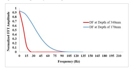
Fig. 4: The Frequency domain of loading pulse on section 1 at 72 km/hr during spring
