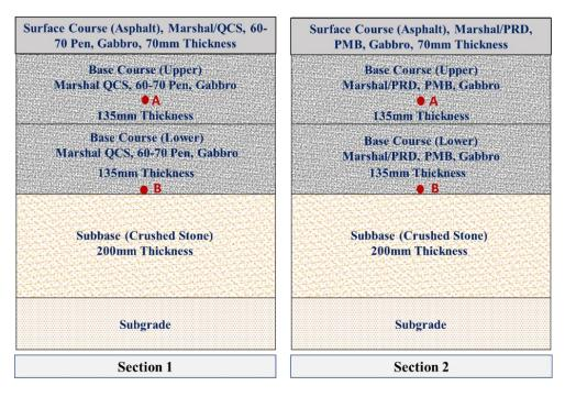
Fig. 1: Layers and Materials' properties of the two selected sections
