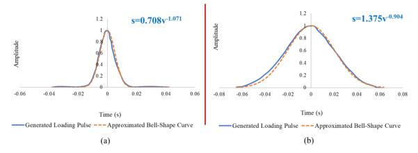
Fig. 3: Normalized Bell-shaped approximations of Loading Pulses for the 72 km/h test applied on section 1 in spring at (a) 170 mm (b) 340 mm
