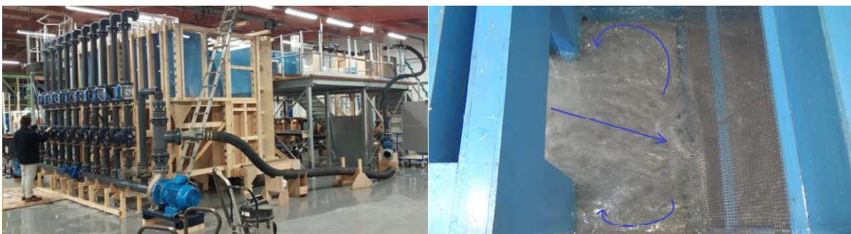
Fig. 8: Model overview and angled jet impinging on the screen
