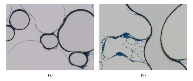
Fig. 1: Microscopic images showing the first flow condition of air drainage, mobilizing the colloids-water suspension from the porous media, (a) hydrophilic collector model with water unfavourable colloids. Similarly (b) hydrophobic collector model with water unfavourable colloids
