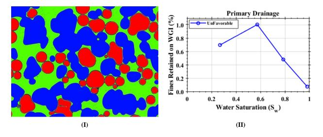
**Fig. 2:** (I) shows a segmented microscopic image of hydrophilic porous media with water unfavourable colloids, phases of gas, water, solid and colloids, are labelled as red, green, blue and grey, respectively. (II) is the measured ratio of colloidal fines retained on GWI to the volume of the porous media, versus water saturation during drainage.
