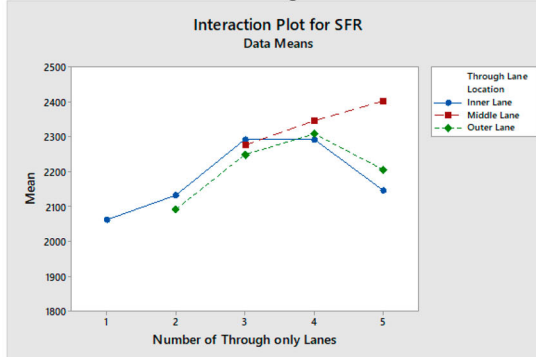
(b) Interaction Plot for Number of Through Lanes and The Lane Location Effect on SFR
