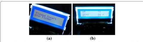
**Fig. 13** The LCD display showing  $\bf{a}$  the message "Please Insert Your Finger",  $\bf{b}$  the  $SpO_2$ , heart rate, and perfusion index for the captured PPG signal
