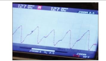
Fig. 10 AC part of the processed PPG signal, captured and processed in the Oxygen Reader Subsystem
