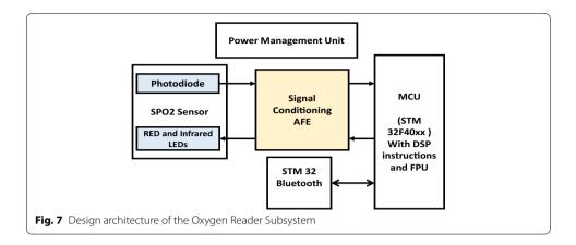
circuit. The transducer circuit converts the low detected current from the photodiode of the  $SpO_2$  sensor to a readable voltage by the microcontroller's A/D. The LEDs driving circuit controls switching operation and the intensities of the Red and Infra-red LEDs of the  $SpO_2$  sensor based on commands from the MCU.
