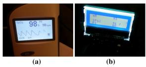
**Fig. 15** SpO<sub>2</sub>, HR, and PI using: **a** commercial Pulse-Oximeter, **b** prototype model for the Automated Oxygen Administration System
