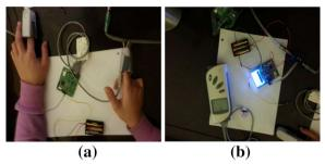
**Fig. 16** Set up for the SpO<sub>2</sub>, HR, and Pl using commercial Pulse-Oximeter and the prototype model for the Automated Oxygen Administration System with its two subsystems that communicate wirelessly: **a** Oxygen Reader Subsystem, **b** Automated Adjustment Oxygen Delivery Subsystem
