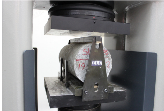
Figure 5. Set-up for splitting tensile strength test.
