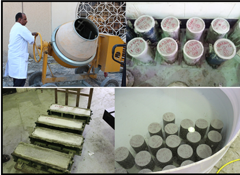
Figure 3. Portion of specimens during mixing, casting, and curing period.
