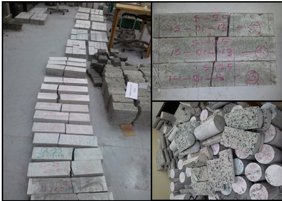
Figure 7. Photos of crushed concrete samples from various tests.
