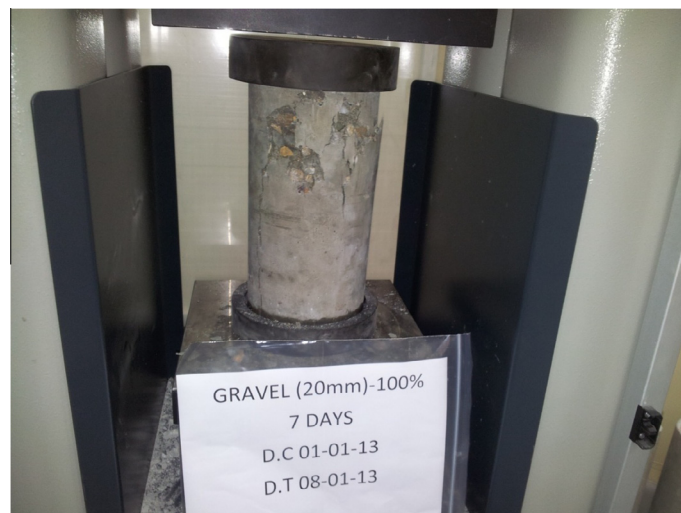
Figure 4. Test set-up for uniaxial compressive strength test.
