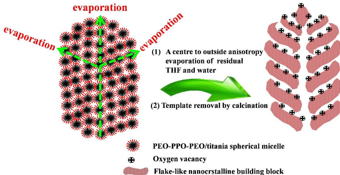
**Figure S21.** Schematic representation of the formation process of curving cylindrical channels within the olive-like mesoporous  $\text{TiO}_2$  mesocrystals through the evaporation-driven oriented assembly process.
