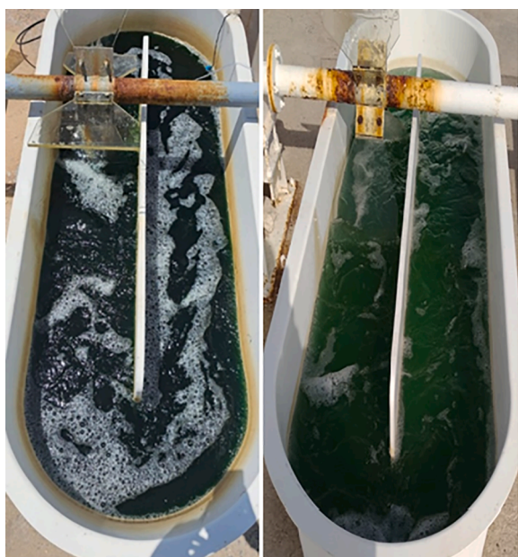
Fig. 2a. Left - Geitlerinema sp. cultivation tank with CO 2 dosing device, Right - Control tank.
