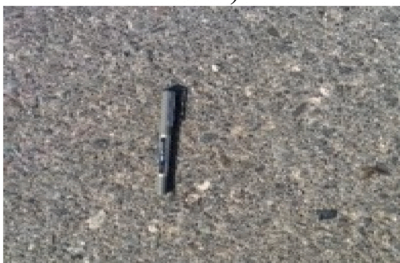
c) Dukhan highway (6 years with NMAS of 19 mm with MTD of 0.88 )
