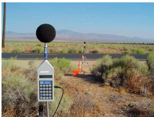
Figure 6. Wayside pass-by measurement apparatus [14].
