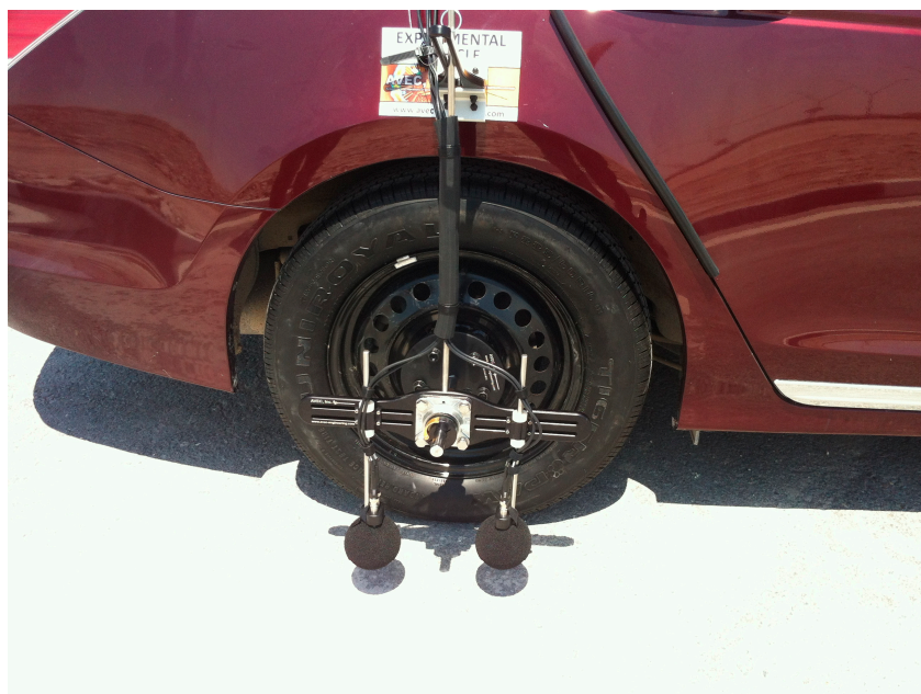
Figure 10. OBSI testing set-up used at Qatar University.
