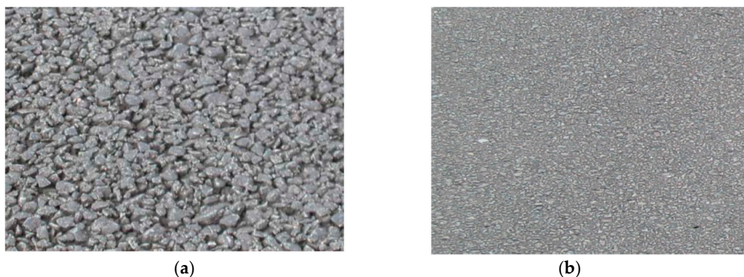
Figure 15. Surface texture of (a) porous asphalt; (b) dense asphalt (Reproduced with permission from European Asphalt Pavement Association (EAPA)) [87].
