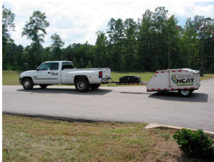
Figure 8. National Center for Asphalt Technology (NCAT) CPX trailer (Reproduced with permission from Hanson et al.) [11].
