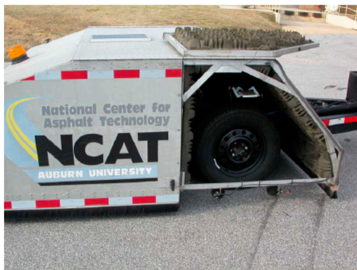
Figure 9. NCAT CPX trailer with across door open (Reproduced with permission from Hanson et al.) [11].
