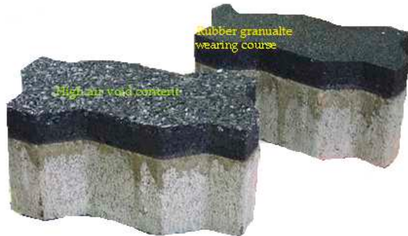
Figure 19. Two types of PERS mounted on interlocking blocks tested in Japan [107].
