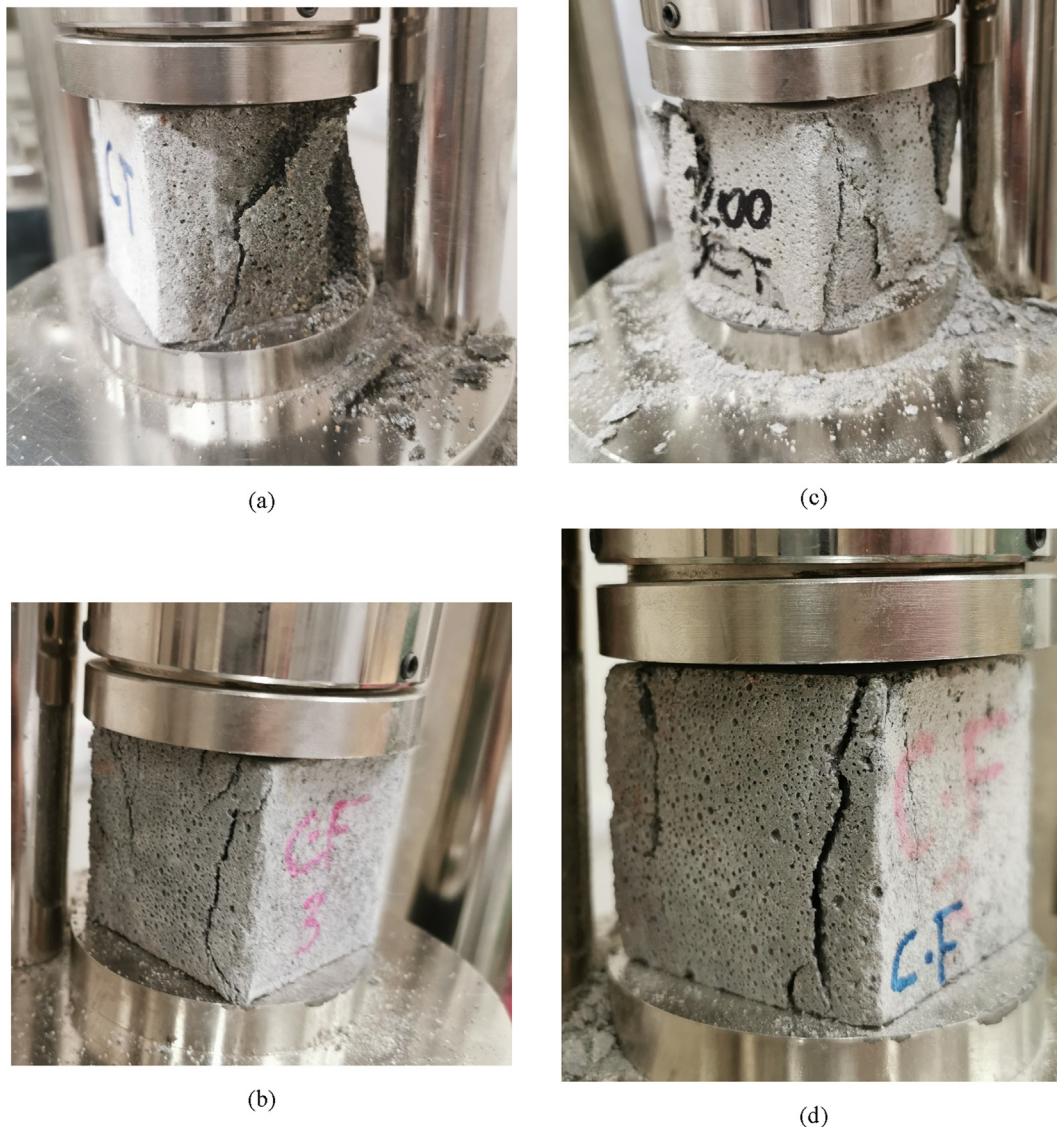
Fig. 4. Typical compressive failure mode of specimens heated up to 450°C (a) plain mortar (b) hybrid-reinforced specimen, and heated at 600°C (a) plain mortar (b) hybrid-reinforced specimen.
