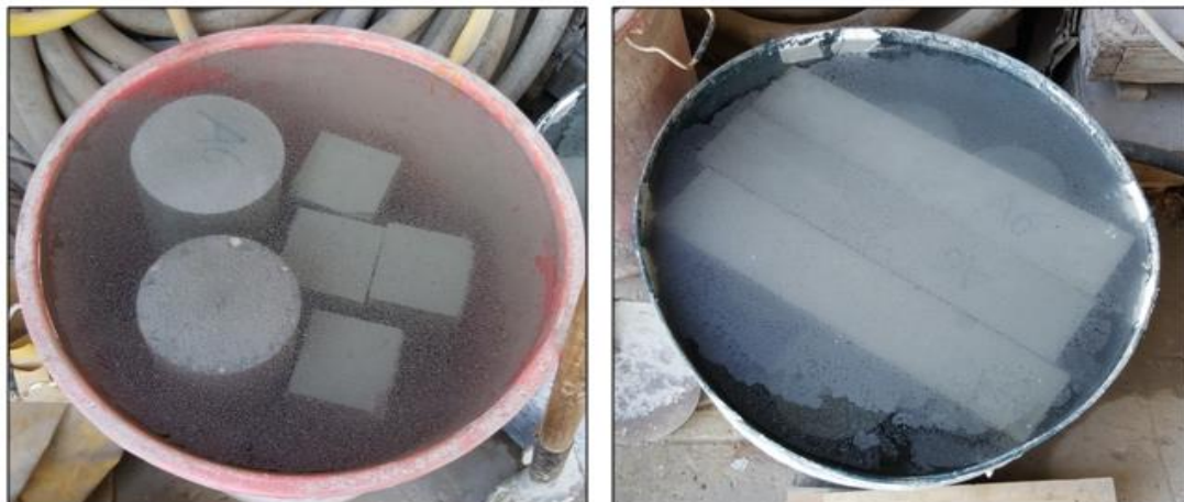
Figure 3.17 Curing of Concrete Cylinders and Prisms
