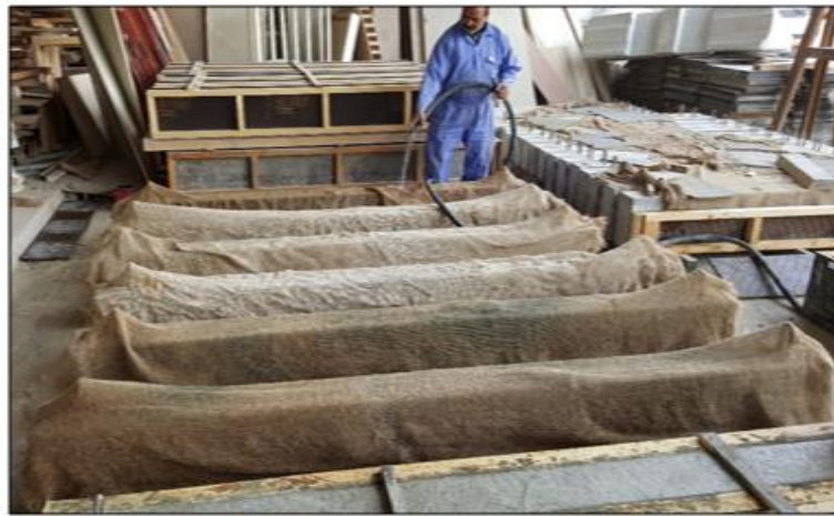
Figure 3.16 Curing of Beam Specimens
