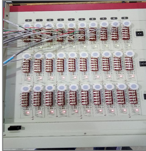
Figure 3.24 Data logger (TML Data Logger Multi-Channel Digital Strain meter DRA-30A)
