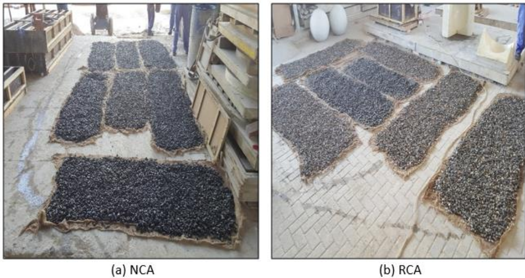
Figure 3.11 Drying the Aggregates to Achieve the SSD Condition
