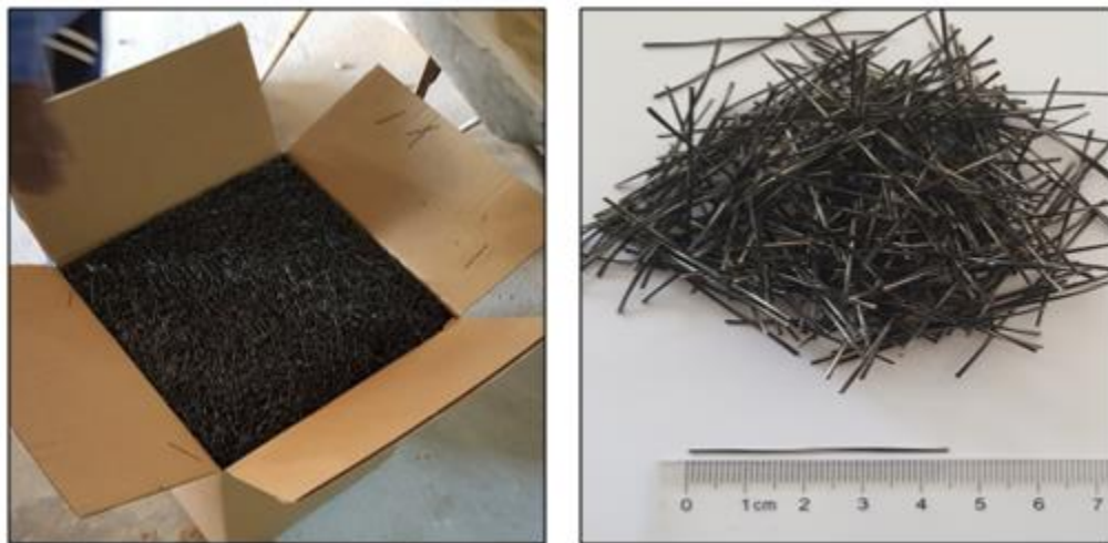
Figure 3.3 Basalt Macro Fiber (BMF)
