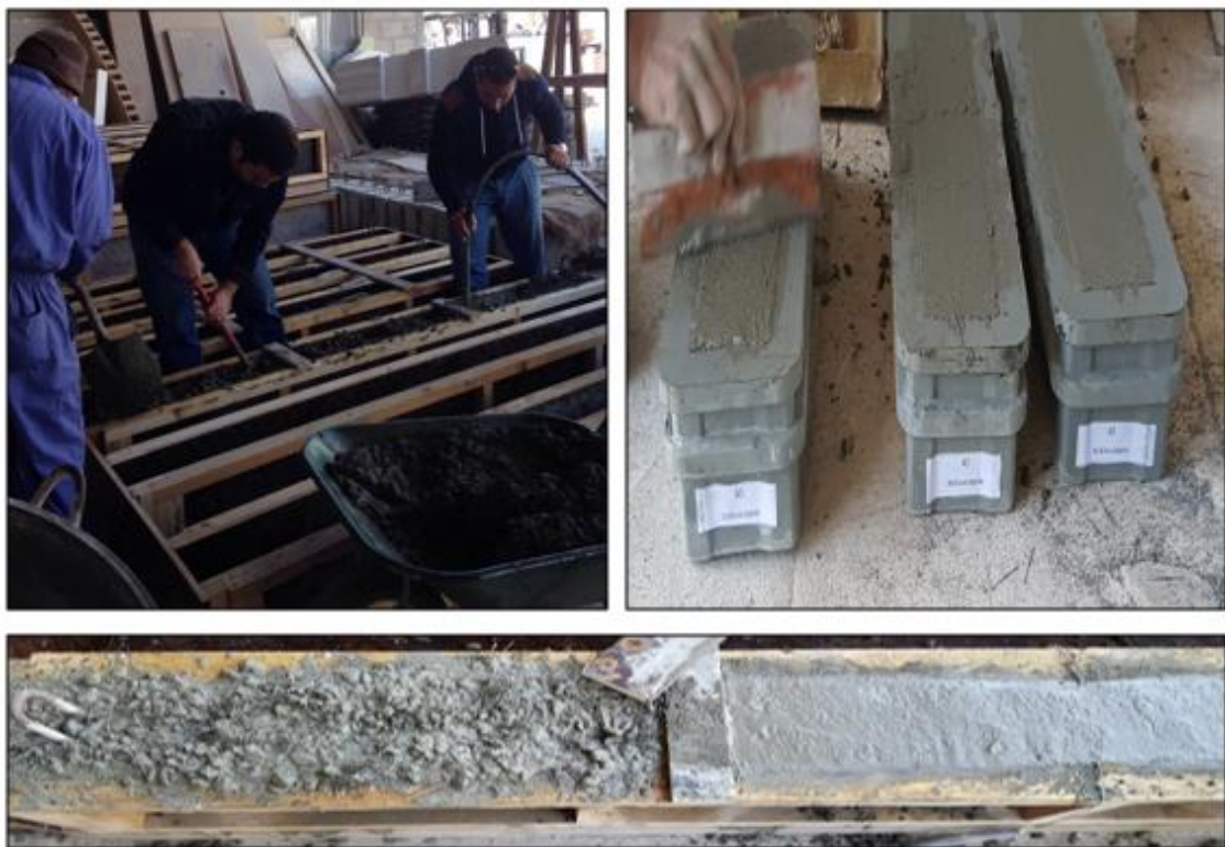
Figure 3.15 Casting of the Concrete Beams
