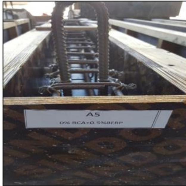
Figure 3.14 Coded Beam Ready for Casting
