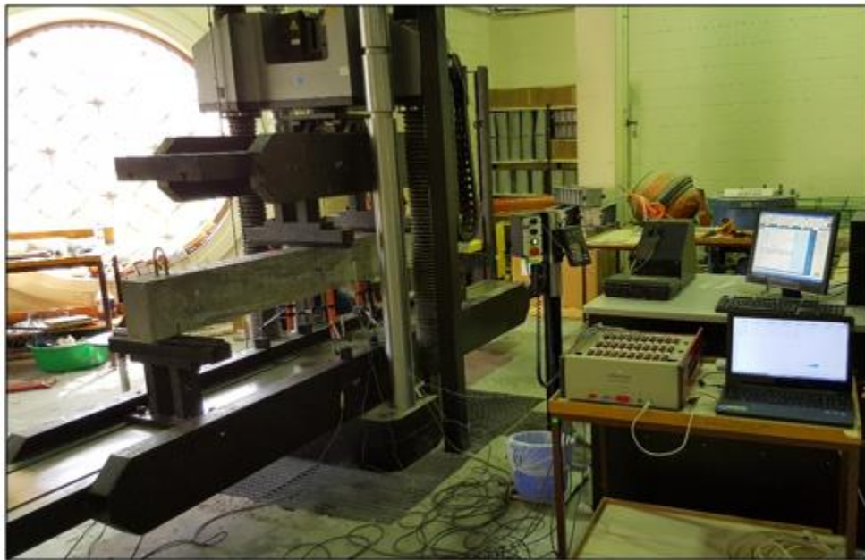
Figure 3.25 Instron 1500HDX Static Hydraulic Universal Testing machine with the deflection transducers and data acquisition system
