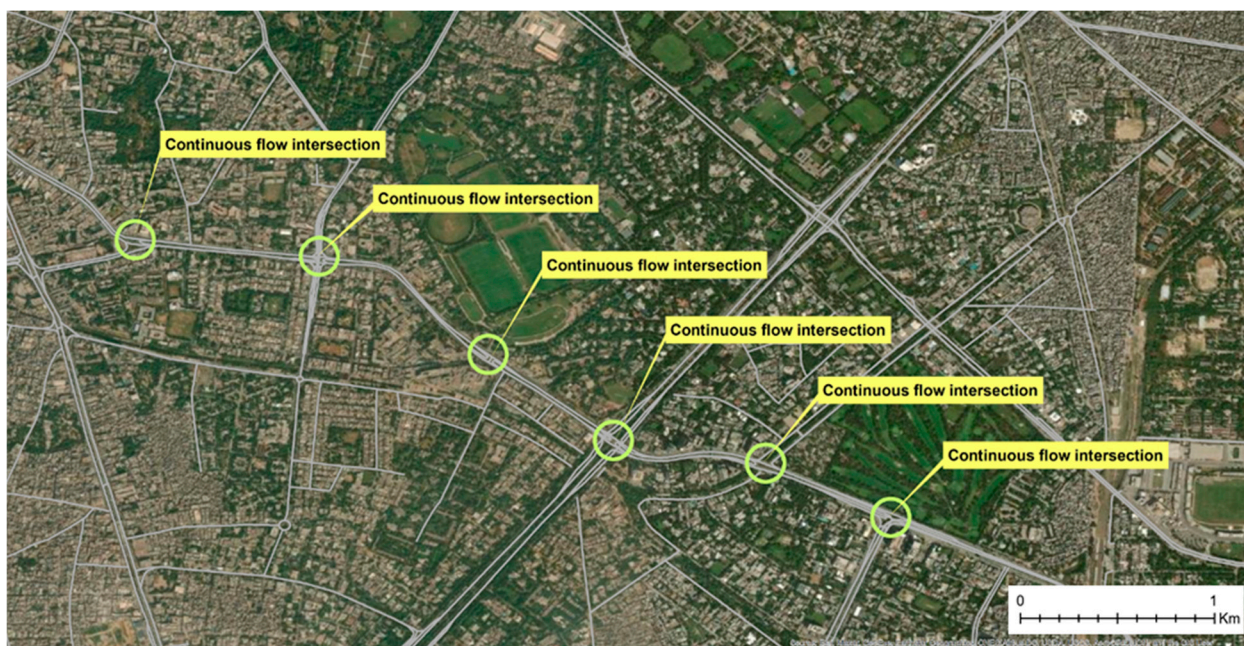
Figure 9. Jail Road SFC created as a result of constructing various CCPs (mainly continuous flow intersections).
