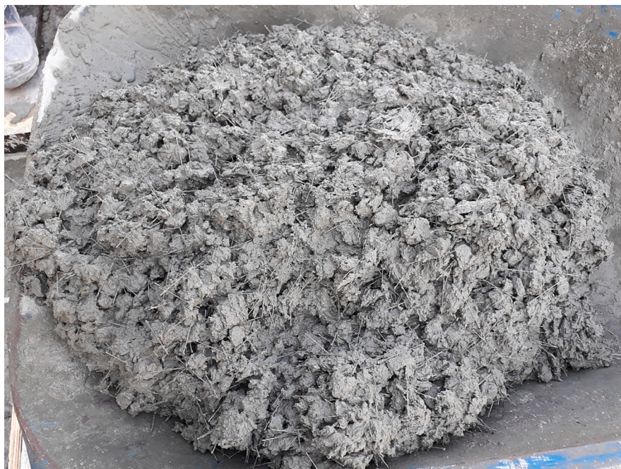
Fig. 8. BMF distribution in the fresh concrete.
