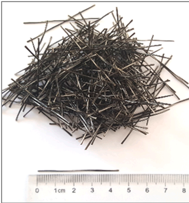
Fig. 3. The basalt macro-fibers (BMF) used in this study.
