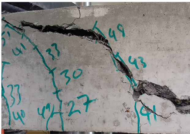
Fig. 6. Bridging effect during testing of beam A-R2-0.75.
