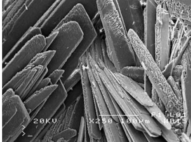
Figure 13: SEM imaging of \text{CaSO}_4 during saline wastewater separation in a DCMD process [56].
