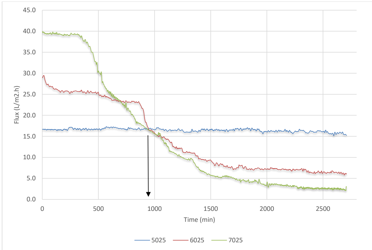
Figure 37: The flux profiles obtained at q_f = 2.5 L/min, where t_f = 50-70 °C, and t_p = 20 °C.
