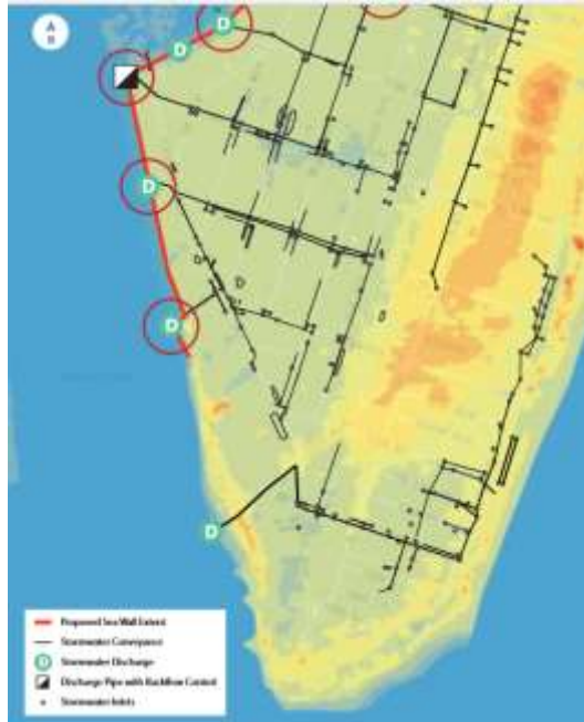
Figure 38. Storm water backflow from discharge points, Source- Evans et al,2016.
