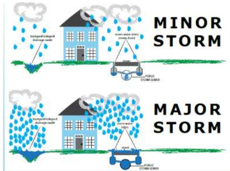
Figure 82: Roads and storm water drains during major storms.
