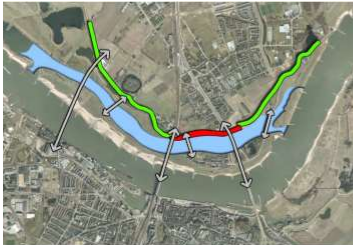
After: The dikes are moved back and a new channel allows more water to flow, reducing flood risk. An island is created in the river, creating room for new development, and new bridges connect residents on both sides of the river. (Room for the River Waal)
