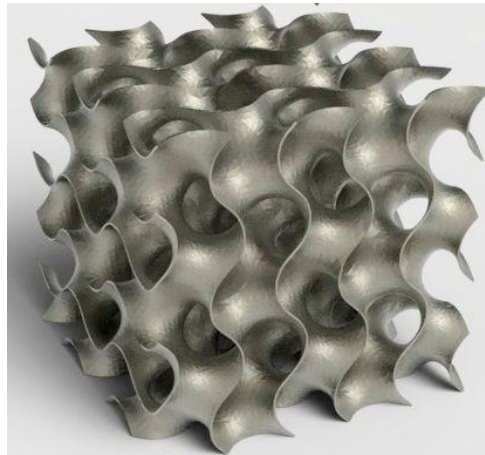
Figure 12. Representation of a 3D model corresponding to a gyroid scaffold [187].
