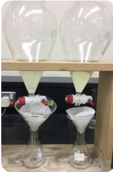
Figure 11: Oil and grease liquid separation process
