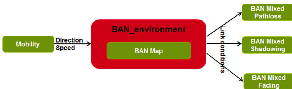
Figure 3. Central position of the BAN environment between the mobility and propagation modules.
