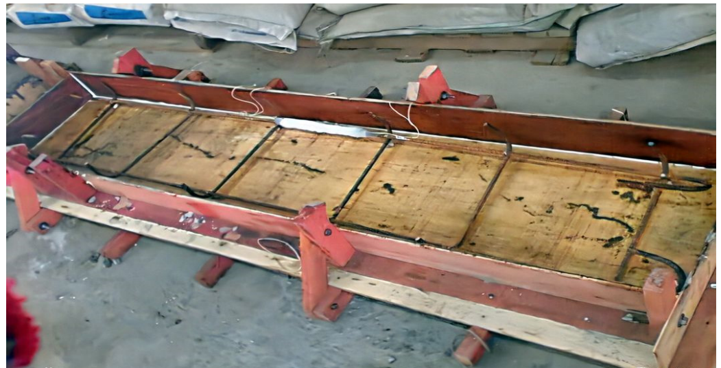
Figure 4. Longitudinal reinforcement utilized in the tested one-way RC slabs.
