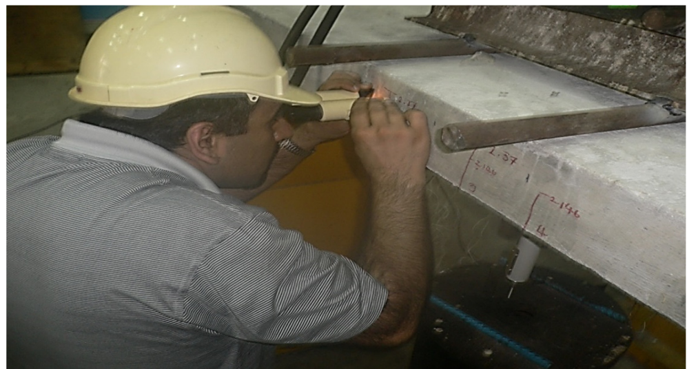
Figure 10. Crack measurement in each stage of the applied load.
