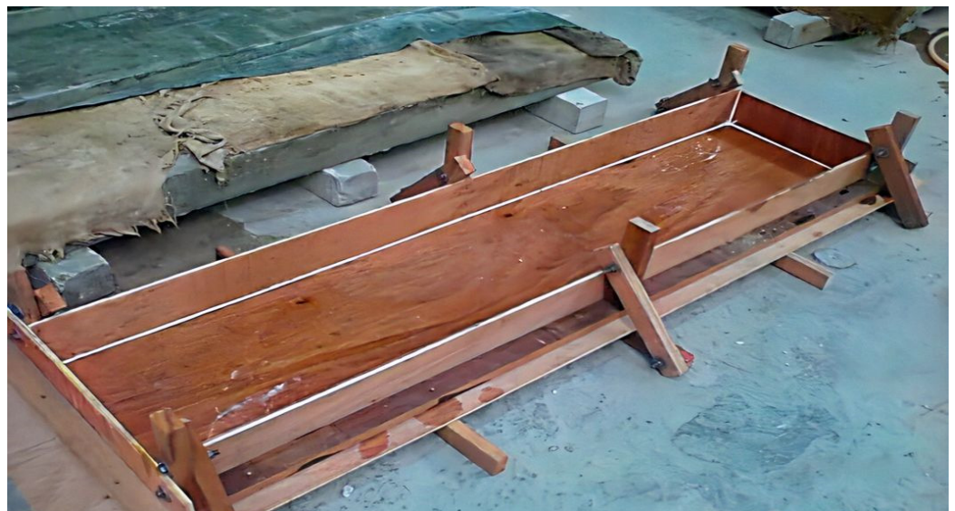
Figure 3. Illustration of wooden formwork for concrete specimen casting.
