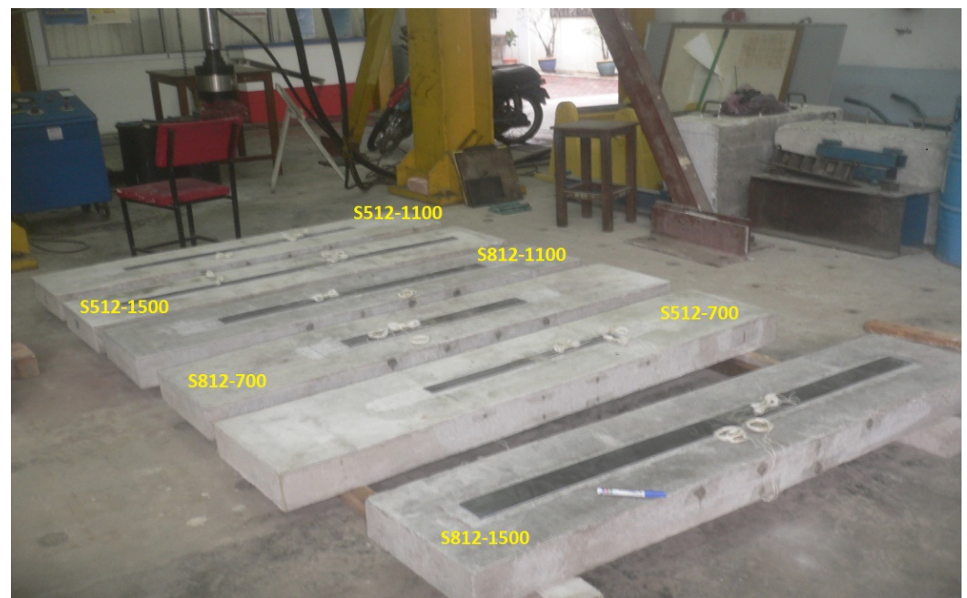
Figure 7. RC slabs strengthened with CFRPs of various lengths and widths.
