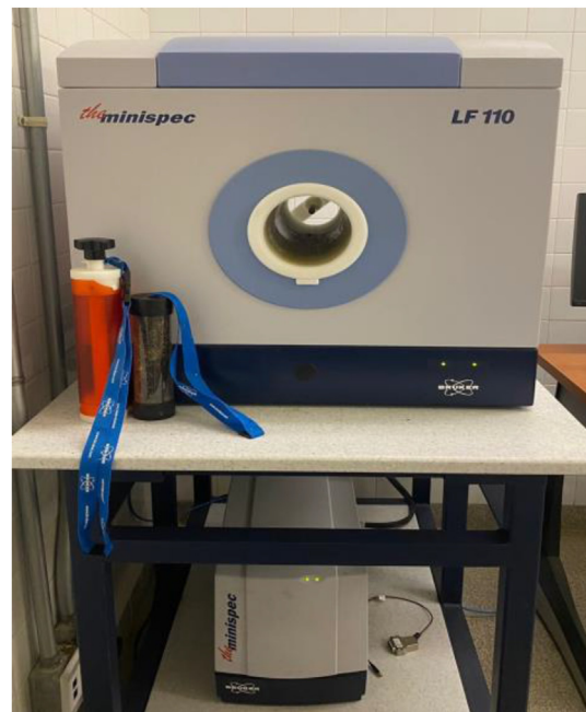
Fig. 2. The LF110 minispec (Bruker, MA, USA) Nuclear Magnetic Resonance Machine. Body fat composition was assessed using the LF110 minispec (Bruker, MA, USA) Nuclear Magnetic Resonance (NMR) Machine. This was done at week 4 (before TBI) and week 8 (after TBI).
