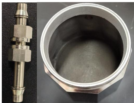
Figure 5. Nitridation reaction column (a) and hydrolysis water container (b)
