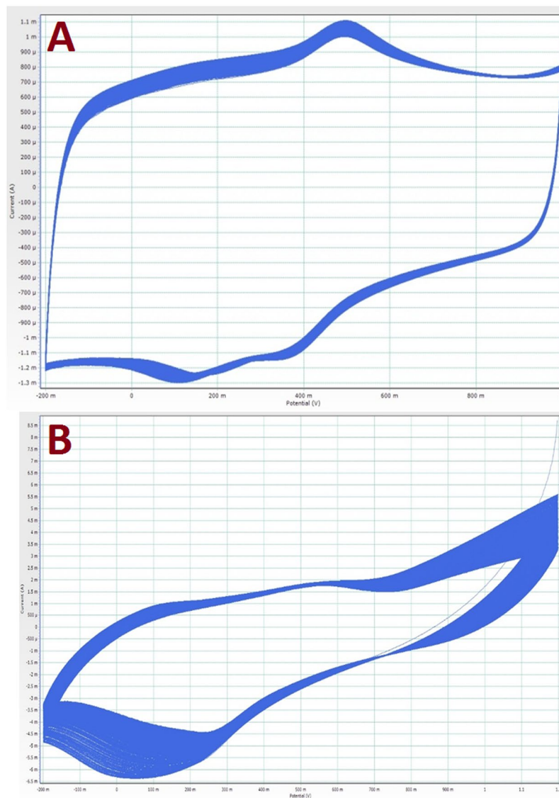
Figure 5. Screen shots for 1000 cycles in 0.5 H 2 SO 4 for the synthesized FeNi-N-Gr; (A) and Pt/C; (B).
